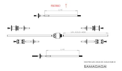
2. Lathe, cut or drill UN AXLE and axle adapter. Join axle with adapter to the demand length and TIG Spot welding. For Axle adapter, Lathe UN AXLE 12.5mm diameter x 40mm to insert axle adapter. For DM adapter: drill 12.5mm diameter hole x 35mm on UN AXLE to join with adapter.
