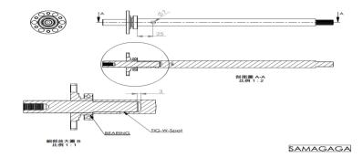
3.Set bearing in proper position and make axle differential alignment (one axle 2 bearings to hold, one close to differential, one close to hub). Axle stopper or pillow block bearing is necessary to hold axle and lock axle does not slide out. We suggest utilizing pillow block bearing and axle stopper to adjust axle differential alignment and fix screw on pillow block bearing after alignment set. IMPORTANT: NEVER HIT AXLE BY HAMMER FROM SIDE WHILE INSTALL AXLE. IT WILL DAMAGE
